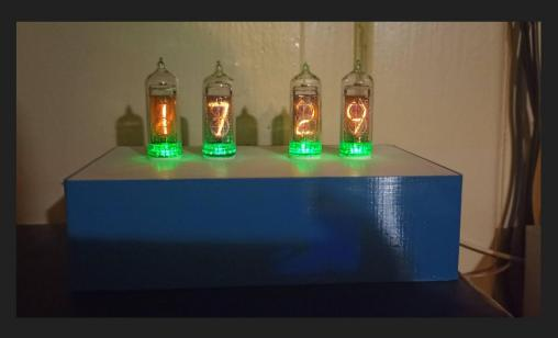
I made a practically identical circuit and used it to power the Nixie ÿÿ-14 tubes (IN-14 after "ours") in the clock.
