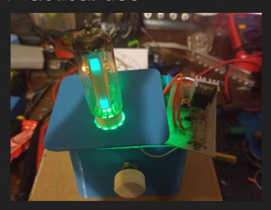
I used this converter to power the "maic eye" 6E2 vacuum tube (EM84 replacement).
