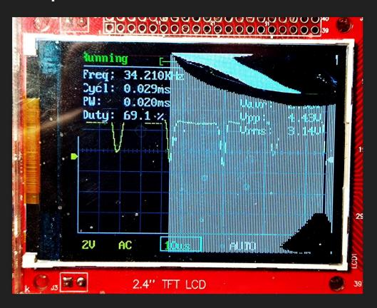
Ignoring the damage to the "toy" screen of the oscilloscope, you can clearly see the waveform that the 555 generates.
