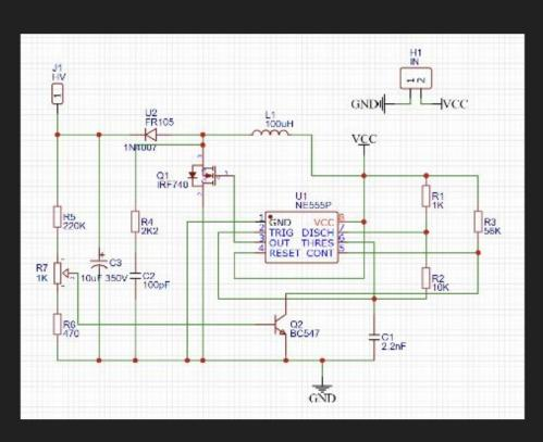
The very popular 555 timer, whose period and duty cycle is controlled by the capacitor C1 and the resistors R1, R2, generates a square wave given to MOSFET Q1.
